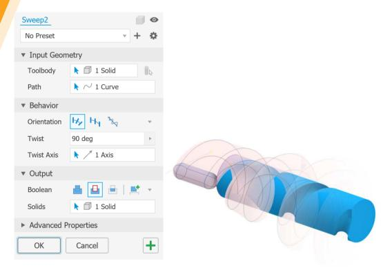
Use a tool body to add or remove geometry in the Sweep command
